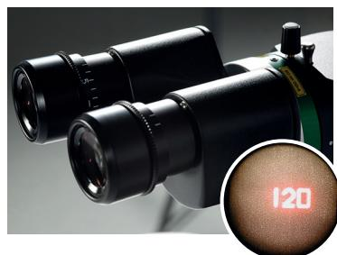
Unique information projection, a feature patented by Valon combined with the Smart Wheel provides complete control of variable values without removing eyes from the oculars. During the treatment the system projects on the retina all customary settings such as laser power, pattern selection, size and rotation.
