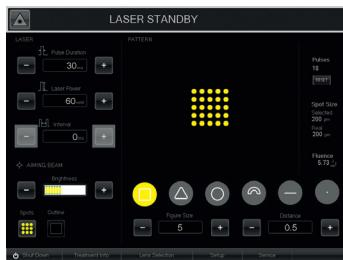
The large and simple user interface provides complete control of all customary settings, such as pulse duration, laser power, pattern selection and pattern size. All parameters are clearly marked with an exceptionally easy access to the Standby/Ready-modes at the top of the screen. The display also shows different automatic reminders built in the system to ensure safe treatment.
